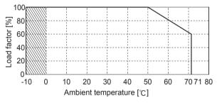
\*In case of ADA600F-24, load factor 100% means output 24V, 21A at ACIN100V, 24V, 25A at ACIN200V.
